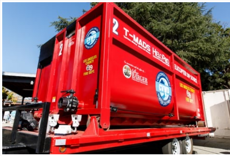
Two water tanks or dip tanks have been provided by CVWD.
